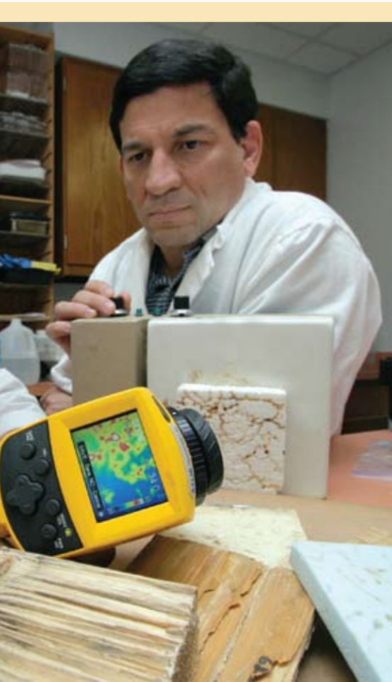
Entomology graduate student Cynthia Tucker, left, and Roberto Pereira, a UF research associate, use a thermal imaging camera to measure heat transfer through building materials damaged by termites. Materials damaged by termites were shown to be less energy efficient, resulting in higher heating and cooling bills.
